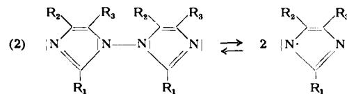
R<sub>1</sub> = R<sub>2</sub> = R<sub>3</sub> = Phenyl:  $k = 0,95 \cdot 10^{-4}$  Mol/l bei 90 °C;  $\Delta H = + 19$  kcal/Mol
